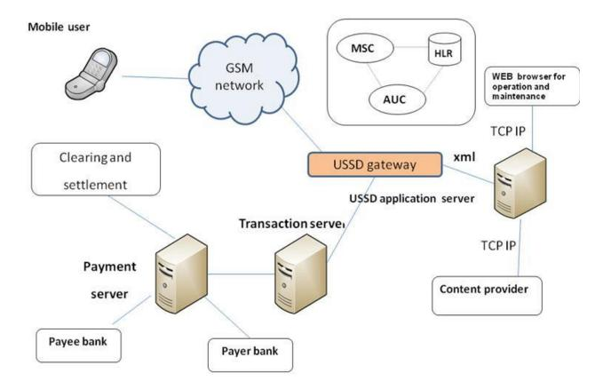
Fig 1: The architecture of mobile payment platform based on USSD [14]
